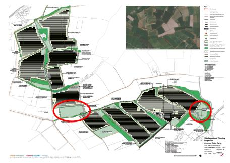
Red circles indicate the areas where panels have been omitted from the proposed site plan
